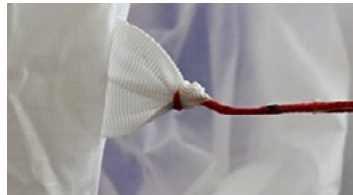
Interlocked junction – correct
