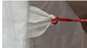
Looped junction – incorrect
